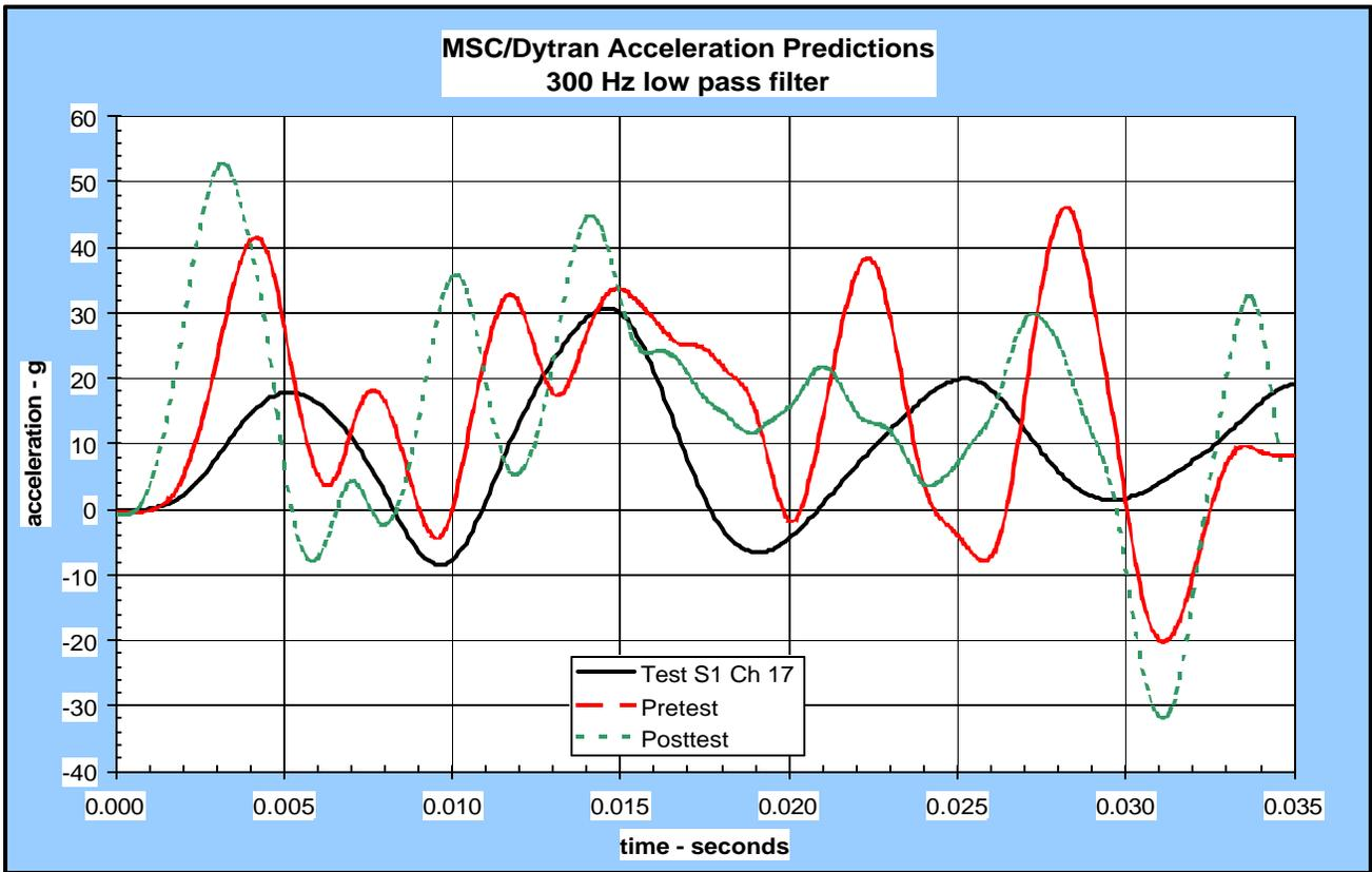
Figure 12. S1 pre & posttest accelerations – FS 155 BL 20 - MSC/DYTRAN vs test
