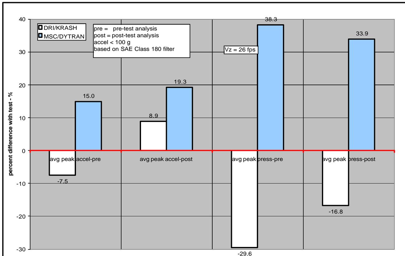
Figure 17. Analysis vs test data - overall
