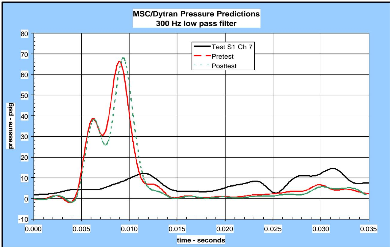
Figure 15. S1 pre & posttest pressures – FS 83.759 BL -1.18 – MSC/DYTRAN vs test
