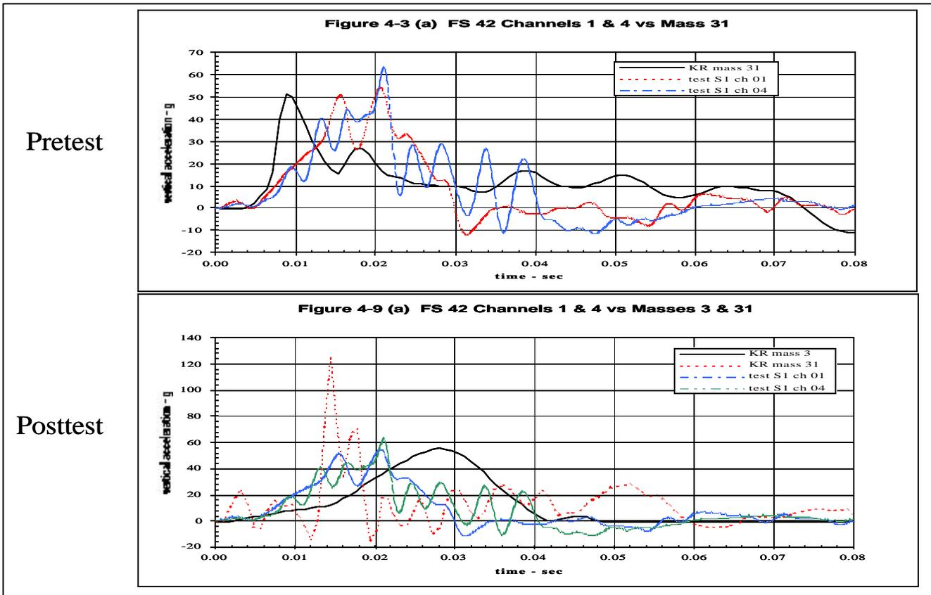
Figure 8. S1 pre & posttest accelerations – FS 42 BL 14 – DRI/KRASH vs test
