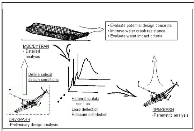
Figure 1. Combined FEM/hybrid approach. Bell Helicopter Textron Inc. (BHTI) developed the MSC/DYTRAN<sup>†</sup> UH-1H Lagrangian model in the manner described below.
