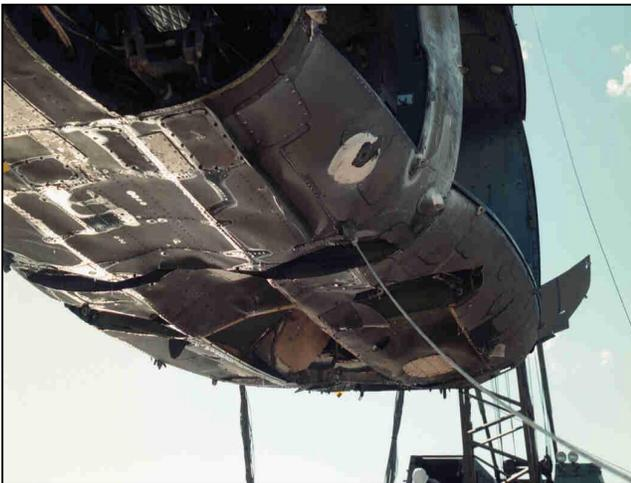
Figure 7. S1 test underside damage
