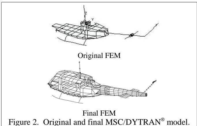
Figure 2. Original and final MSC/DYTRAN<sup>®</sup> model.
