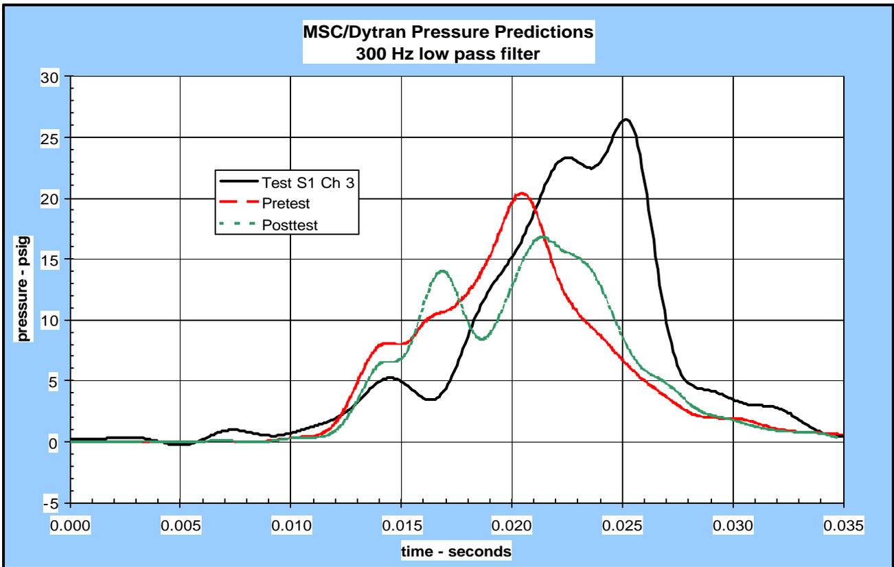
Figure 13. S1 pre & posttest pressures – FS 45.25 BL 23.25 - MSC/DYTRAN vs test
