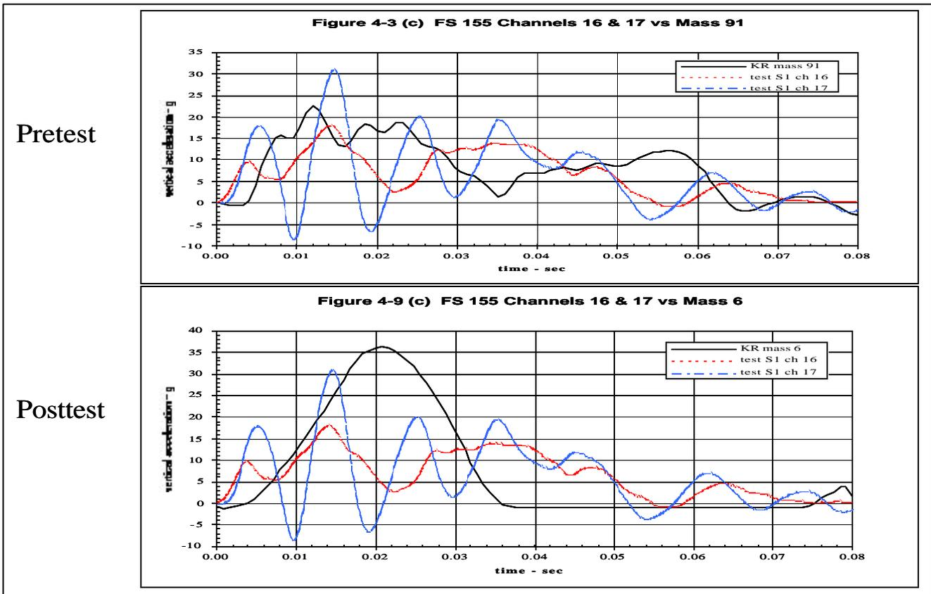
Figure 9. S1 pre & posttest accelerations – FS 155 BL 14 – DRI/KRASH vs test
