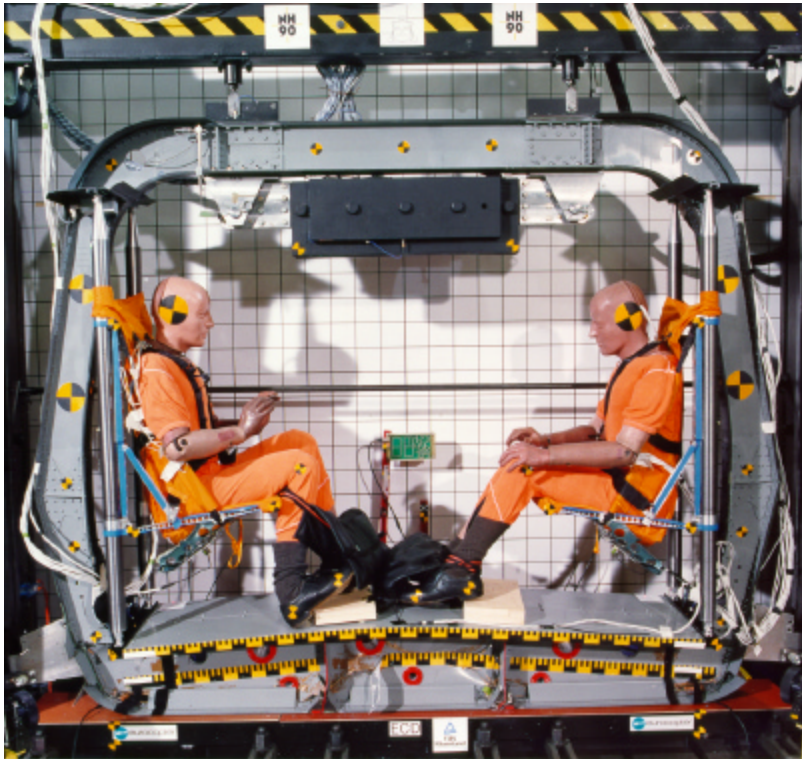
Figure 4 Drop-Test of NH90 frame #6 in 1998
